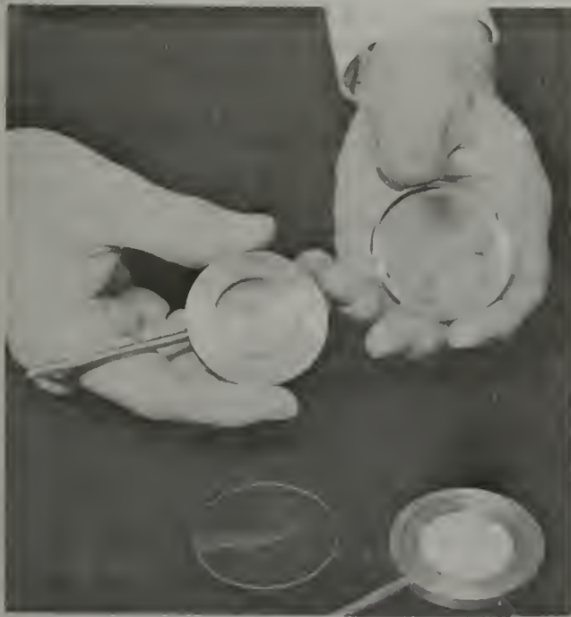
FIGURE 3. Preparation of an opaque powder sample for comparison with the Munsell color scales.
